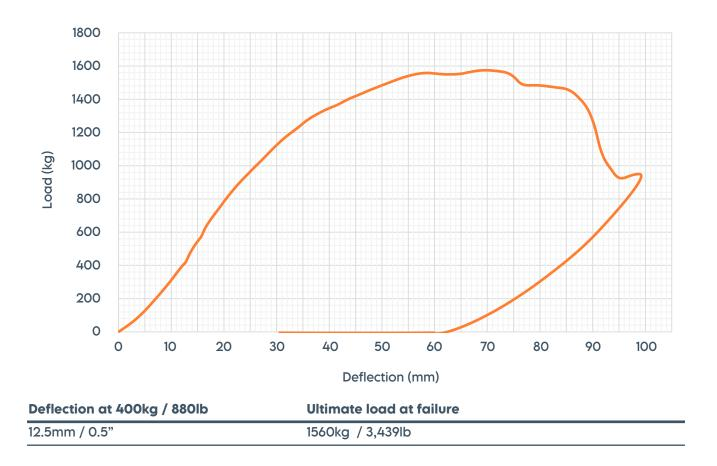
Destructive testing has been carried out on the product to simulate deflection under the working load, and ultimate failure.
