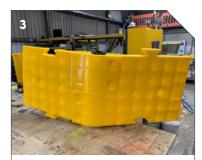
Retrieve two Bypass Ramp Halves and lay them on their side, ensuring they slot together. Front as shown.
