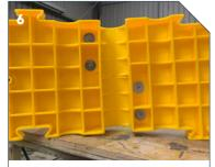
Using another M 8 x 50 washer and an M 8 nyloc nut, fasten this from the underside hand-tight.
