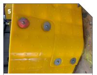
Place an M 8 x 50 washer in the recess on the top face of the Bypass Ramp and insert an M 8 x 30 socket button head screw through from the top face side.
