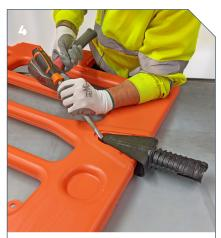
Hammer the screwdriver down into the spigot until the spigot comes loose and remove it.
