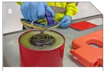
Clean the recessed reflective surface area with a new cleaning sponge soaked with the Alcohol and allow to air-dry for 15 seconds.
