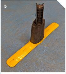
Insert the new spigot into the new foot and place on the floor.
