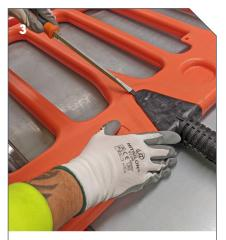
Insert the flathead screwdriver at the apex of the spigot, at a 45 degree angle.
