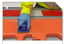
Use a new sponge coated in Standard Primer and, starting at the bottom, ensure that the primer has covered and wetted the whole area. Leave to air dry for 5 minutes.
