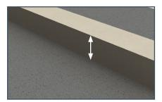
Confirm kerb height suitable: 60mm / 2.4" to 160mm / 6.4".
