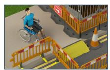
Ensure barriers are set up to leave a minimum of 1m unobstructed space, preferably 1.5m / 4.9ft between ramp and barrier for wheelchair and scooter users.
