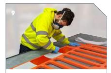
There should be no cuts or tears in the reflective. Air bubbles should not exceed 5x15mm or 10x10mm. Air bubbles should be no closer than 20mm to the edge.
