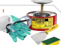
You will need a wallpaper scraper, sponges, a self-made applicator, a plunger can filled with PA Isopropyl Alcohol, a plunger can filled with standard CP906-P1 Primer and PPE.
