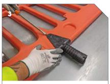
Insert the flathead screwdriver at the apex of the spigot, at a 45 degree angle.
