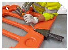
Hammer the screwdriver down into the spigot until the spigot comes loose and remove it.
