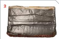
The applicator should be a handheld size, approx. 12x8cm. Fabricate from a piece of hard plastic or card, wrap this in felt, wrap this in a tough fabric and secure together with duct tape.
