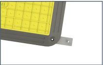
3. Insert the plates underneath the LowPro through the bolt hole.
