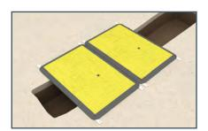
4. Place the LowPros with the plates centred over the width of the trench.
