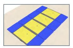
7. Continue placing LowPros over the trench & attaching Infills until the trench is fully covered.
