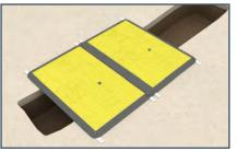
5. Place the Infill between the LowPros, fix Infills with bolts.
