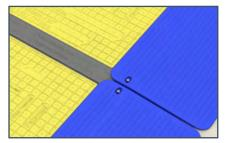
6. Place the Ramps onto the studs on the Plates, and fix Ramps with Bolts.
