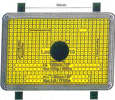
Figure 2: Test load footprint and location
