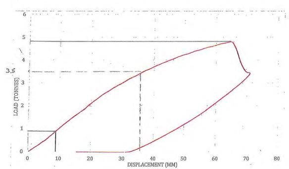
Figure 4; Test Results 15/10 LowPro Load vs. displacement
