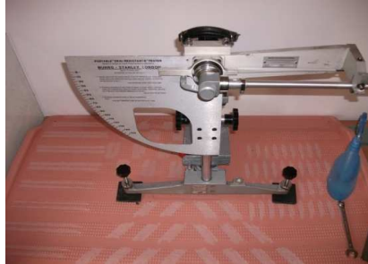
Image 1. Pendulum tester in-situ
