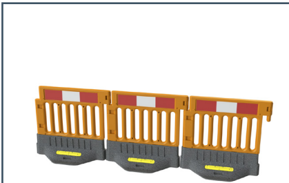
Insert the next StrongWall top so that the connecting pin slots into the locator hole of the previous base.
